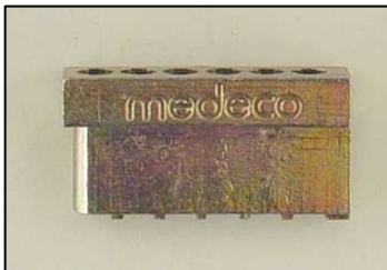
Figure 6, 7, & 8: Pinning tool, new spring cover/retainer, spring cover being removed.
